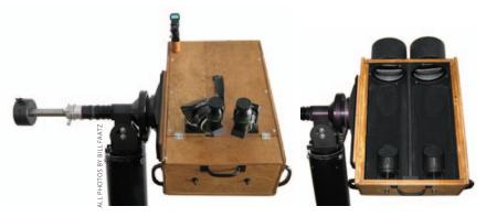
Each half of the binocular uses a pair of star diagonals — a 2-inch model and a 11/4-inch that holds the eyepieces. Inter-ocular spacing and rough focusing is done with helical focusers, while fine focus is achieved by sliding the eyepieces in and out of the star diagonals.
