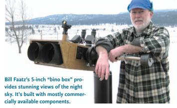
reports, "The helical focusers allow inter-ocular spacing adjustment of the eyepieces, and the star diagonals provide a 90° viewing angle."
